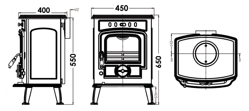
\*All measurements in millimetres (MM) All Dimensions are correct at time of publishing, but may be subject to slight change. Please confirm exact dimensions before comemencing installation works
